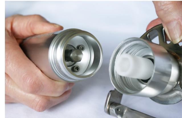
To reassemble, first align the coupler to the drive shaft and push together to engage before screwing the head back onto the handle.
