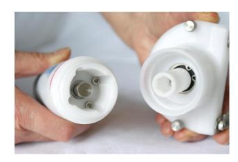
To reassamble, first align the coupler to the drive shaft and push together to engage before screwing the head back onto the handle.
